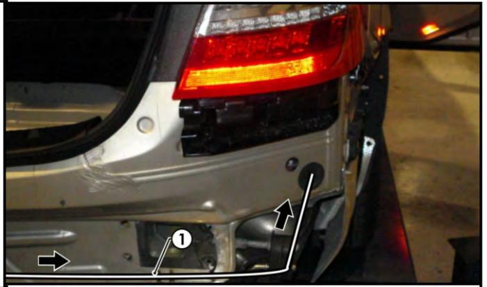
30. Connect the tail harness (tail length 1200mm) 8-way connector (1) to the trailer harness mating 8-way connector (2).
