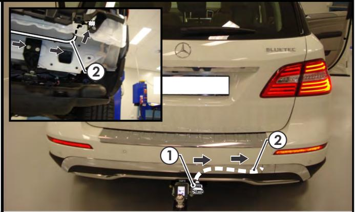
25. Connect the tail harness (tail length 1200mm) 8-way connector (1) to the trailer harness mating 8-way connector (2).
