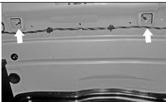
Figure 6 – Remove screws inside panel.
