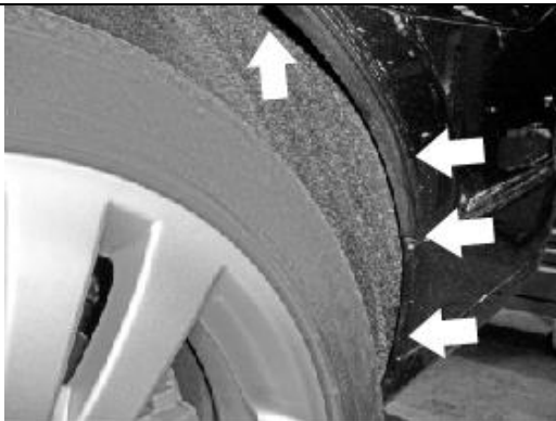
Figure 2 – Remove scrivenets, nut and bolt from wheel arch.
