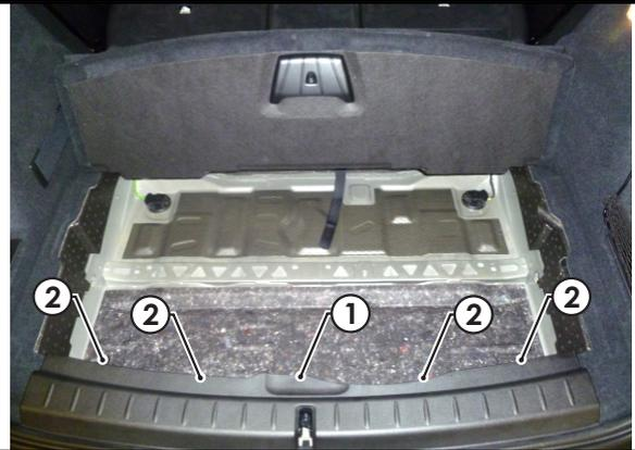
4. On the RHS luggage compartment trim (1) remove the three torx screws (2) from underneath the tie-down caps (2). Dislodge the trim (1).
