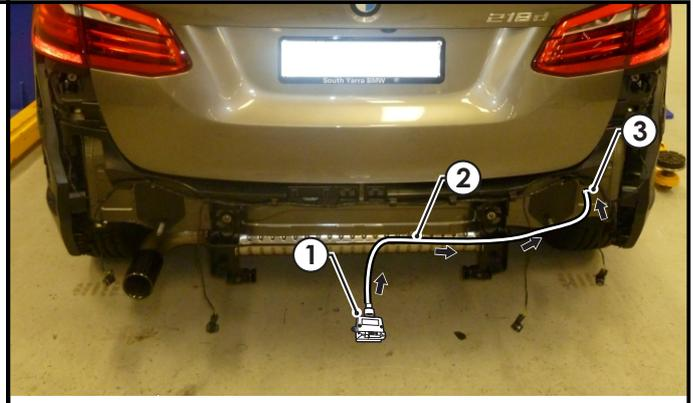
19. Connect the tail harness 8-way connector (1) to the trailer wiring harness mating 8-way connector (2).
