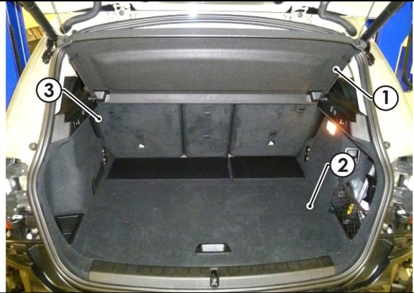
3. Remove the luggage compartment rear trim (1) by removing four clips (2).
